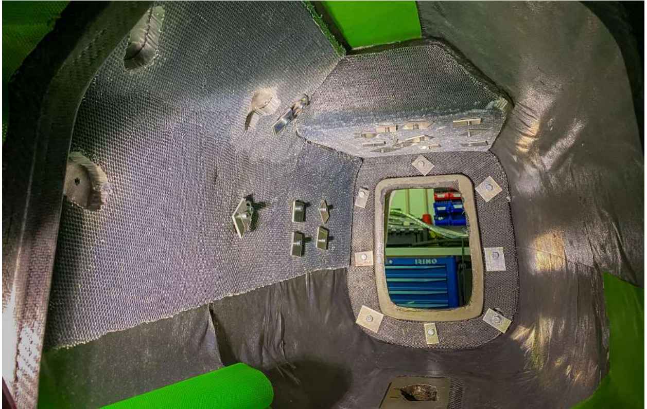
Figure 42: Honeycomb Aluminium provided by Goodfellow reinforcing the FST 10e's monocoque.
