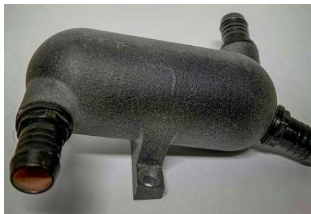
Figure 45: Reservoir of the FST 10d's water cooling circuit printed in PA 12.
